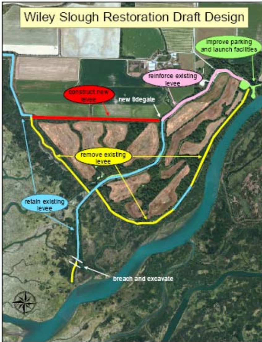
Figure 3-4 Wiley Slough Restoration Design
