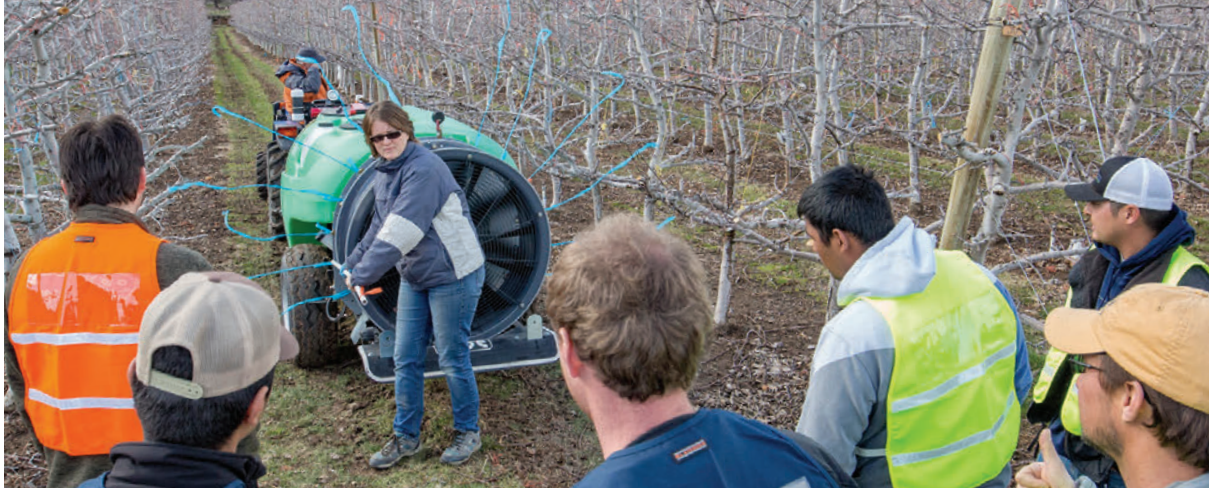
Hoheisel shows how to check the direction of an orchard sprayer's nozzle by using ribbons attached to each nozzle
