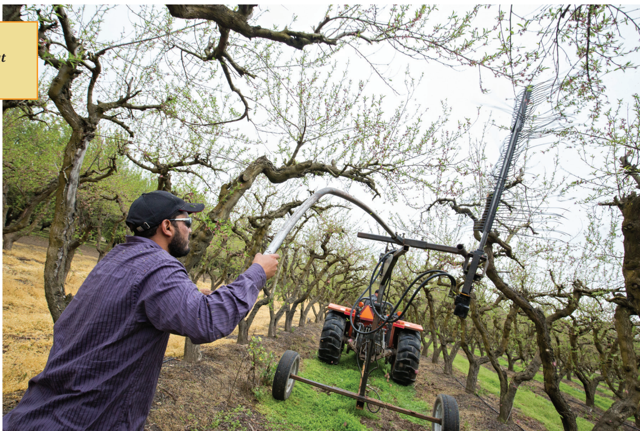
Adrian Rey operates the modified thinner on a pivoting arm, which makes it easier to swing the strings and follow the contours of the canopy.
