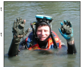
Figure 3. DGER geologist Chris Johnson dives for pond-bottom sediment samples. Diving to collect samples is more work, but provides a better quality sample.
