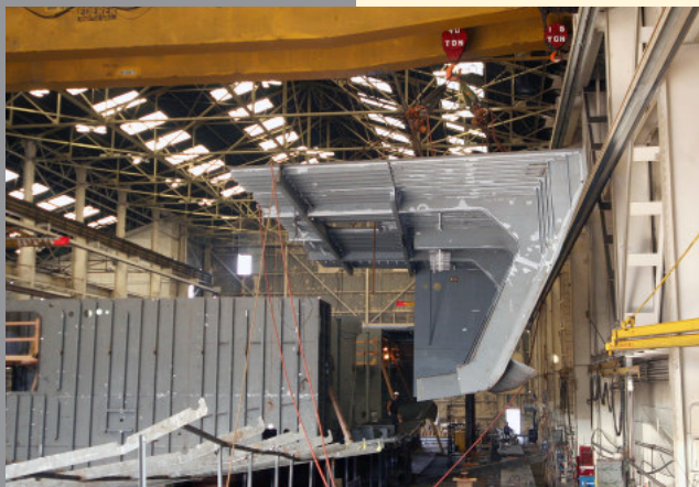
Cranes lift the 26-ton side shell assembly into place.
