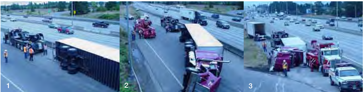
The photo sequence above shows the MIT program in action: Photo 1 shows a class S-1 tow truck preparing to move the fully loaded, rolled-over semi. Photo 2 shows the tow using cables to pull the truck from the middle of the interchange towards the side of the road. Photo 3 shows the semi fully removed from the road. The interchange is once again open to traffic, and crews can begin unloading the cargo in a safer environment.
