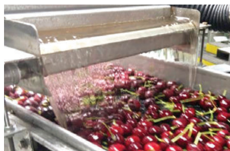
Cherry line with waterfall application of a protective coating.
