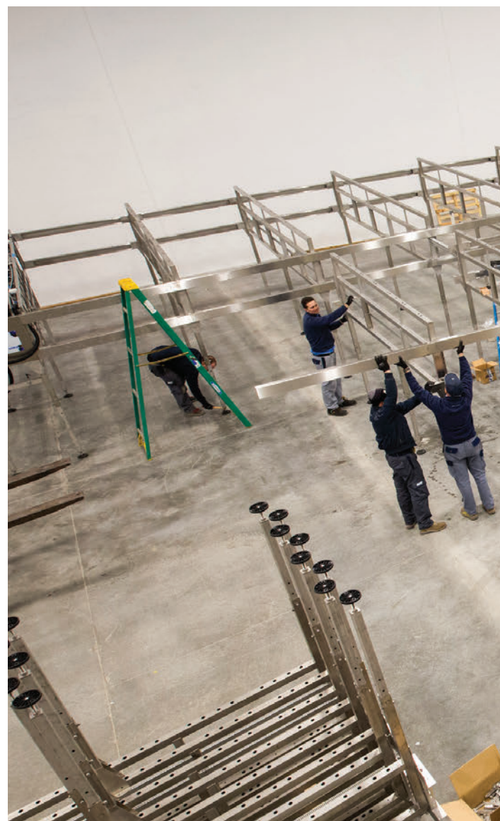
Workers install a cherry processing line that will feature optical
