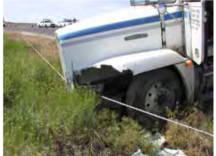
A semi-truck enters the median and encounters cable median barrier head-on – and is successfully stopped.
