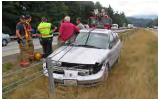
Automobiles trapped in cable barriers tend to remain in the median, rather than rebounding into traffic or entering the opposing lanes.
