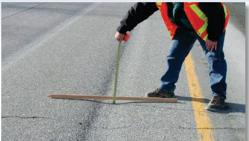
Studded tires have eaten away the asphalt pavement creating these ruts on I-90 near the Idaho border.
