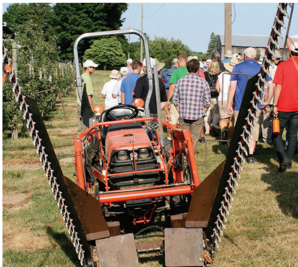
A two-row hedger, designed and built by Paul and Walter Wafler to run down their 7-foot rows between their tall spindle tipped trees, is able to hedge two rows at a time. The machine cuts labor time and costs in half for this task.
