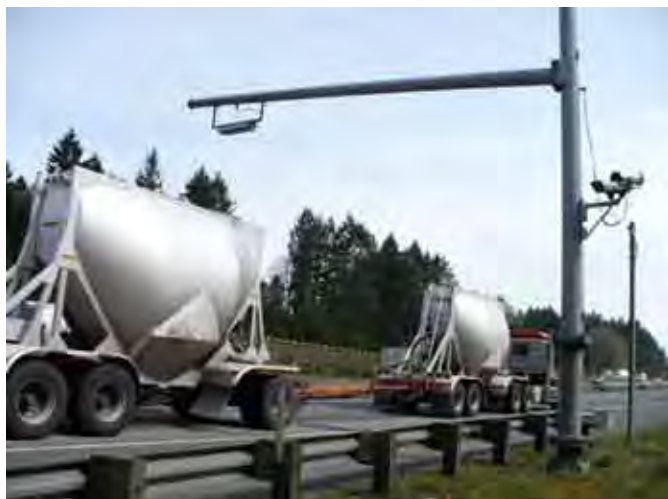
Automatic Vehicle Identifier (AVI), weigh-in-motion scale (WIM), and camera, near Fort Lewis weigh station.
