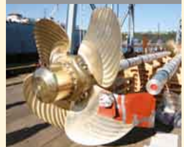
Controllable pitch propeller and tail shaft for the second Kwa-di Tabil Class ferry, Salish .
