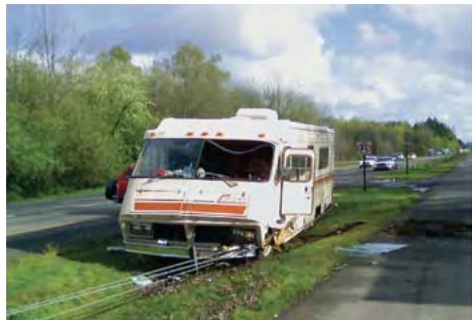
This RV found itself tangled up in cable barrier, which kept it from both rebounding back into traffic and running through into oncoming traffic.
