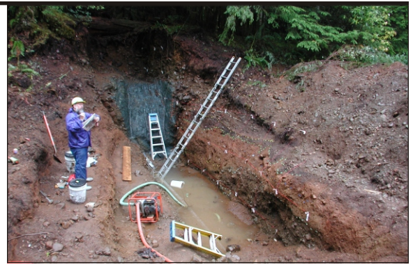
Figure 2. Geologist Tim Walsh logs a trench across the Canyon River fault. Note the use of flags and nails as position markers.
